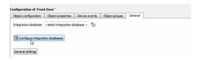
**Note**: Each integrated device needs to be attached to an integration database. Without setting up/adding a database here, the integration will not function properly within the CathexisVision system.
