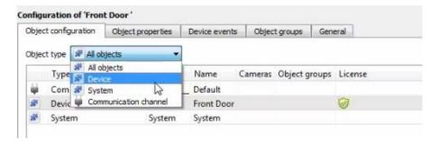
All Matrix COSEC objects (for Device, System, and Communication channel) are automatically populated when communication to the Matrix COSEC Server is established. It is not necessary to add new devices/readers manually.
